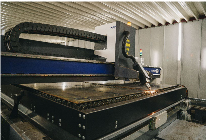
Image 1: The ELEMENT L laser machine scores points with its high dynamics, state-of-the-art laser technology and the ability to process XXL sheets economically.
