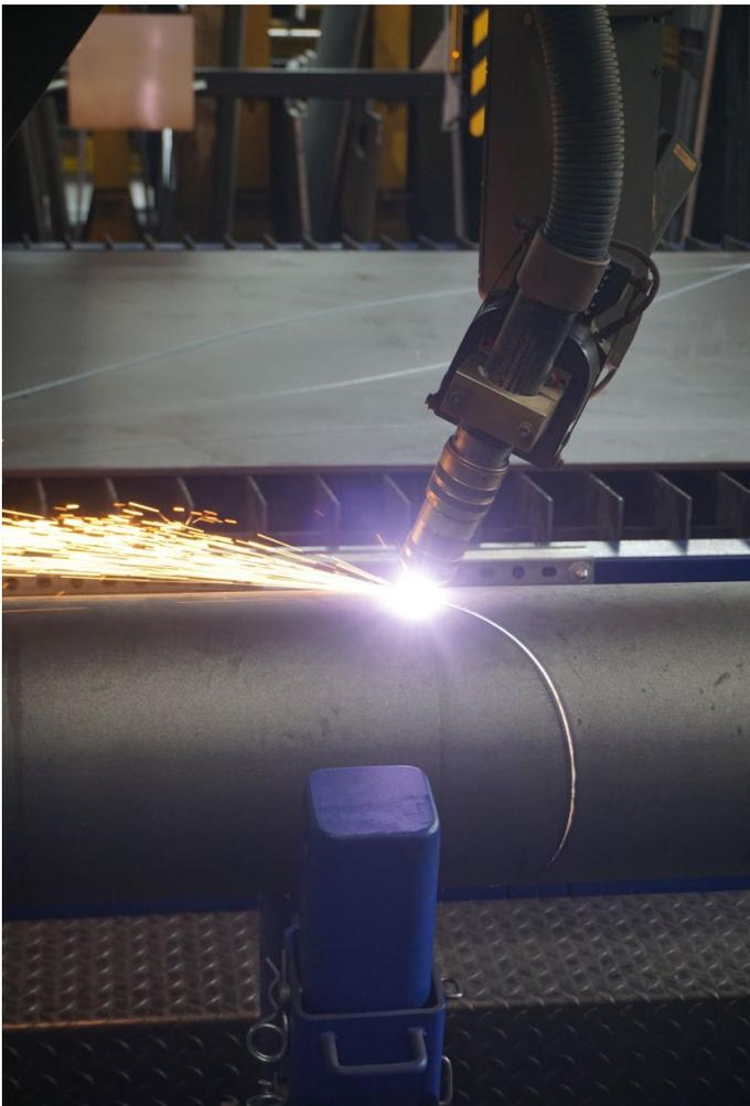
**Caption 4:** The PTC500 pipe cutting system can be used to process round pipes with a diameter of up to 500 mm. The Skew Rotator Delta ensures precise bevel cuts for weld seam preparation.
