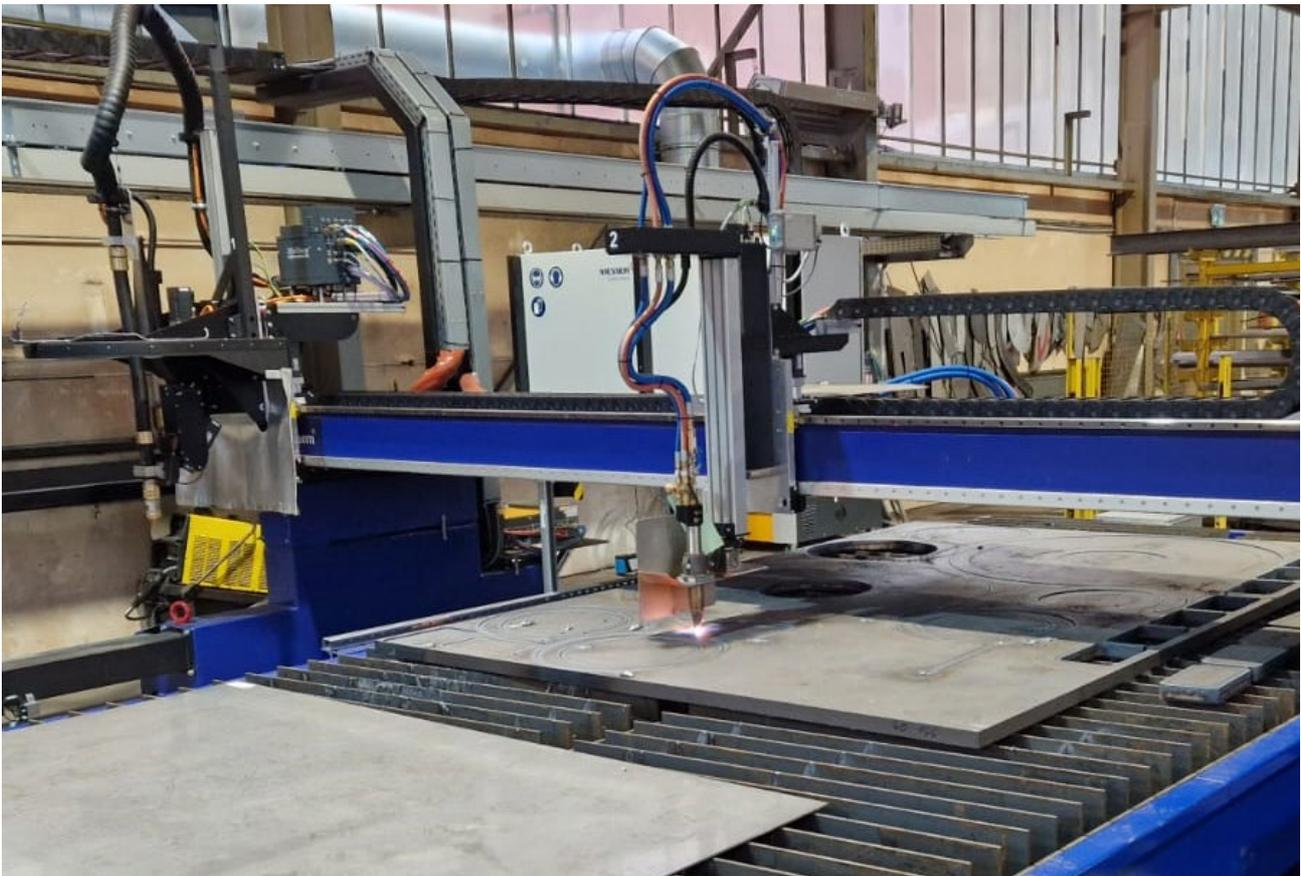
**Caption 5:** The ALFA oxy-fuel torch cuts effectively right to the edge of the plate, ensuring better material utilisation. © Thöni Industriebetriebe GmbH
