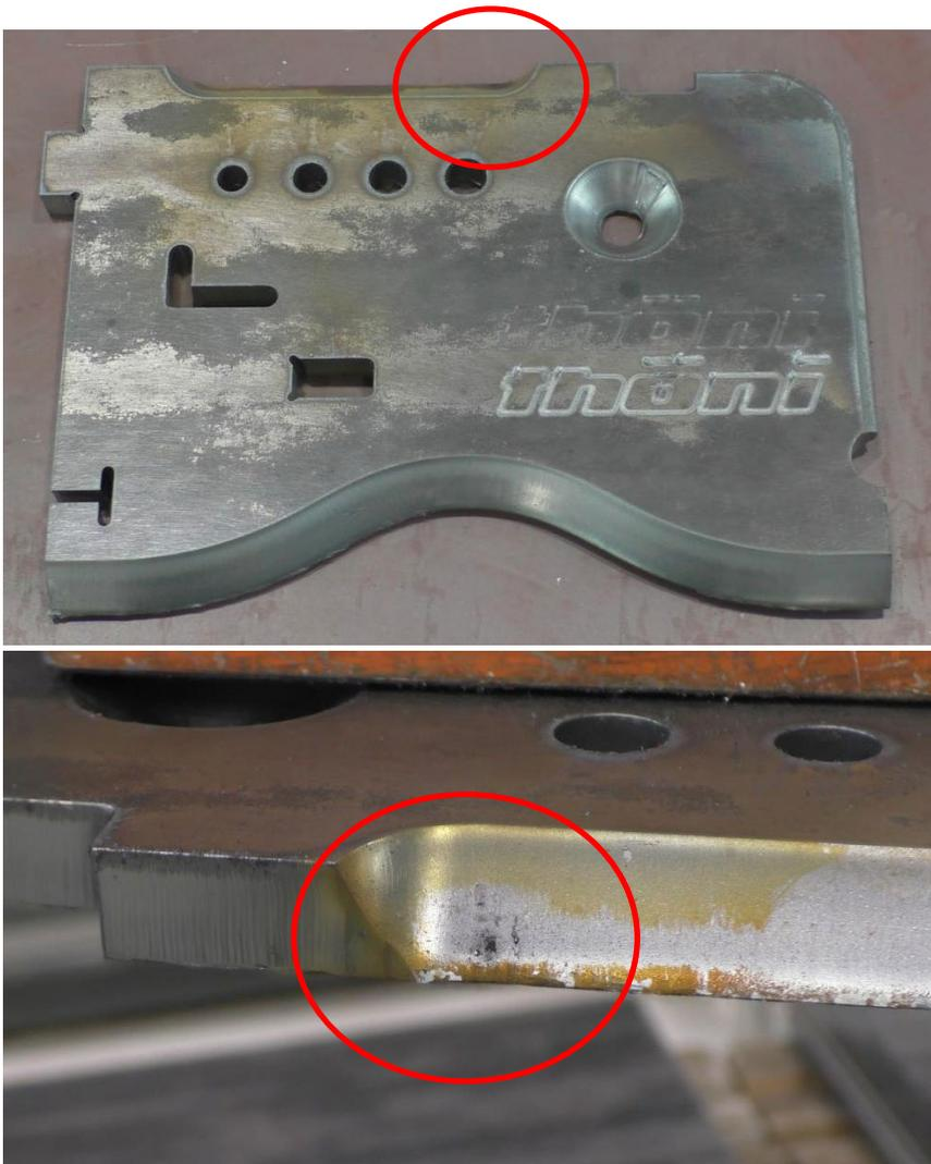
**Captions 7 + 8:** Saves time and costs: Thanks to the Skew Rotator Delta, holes and bevel cuts can be produced directly on the machine and no longer have to be milled or drilled. (Picture below: VDS cut), © Thöni Industriebetriebe GmbH
