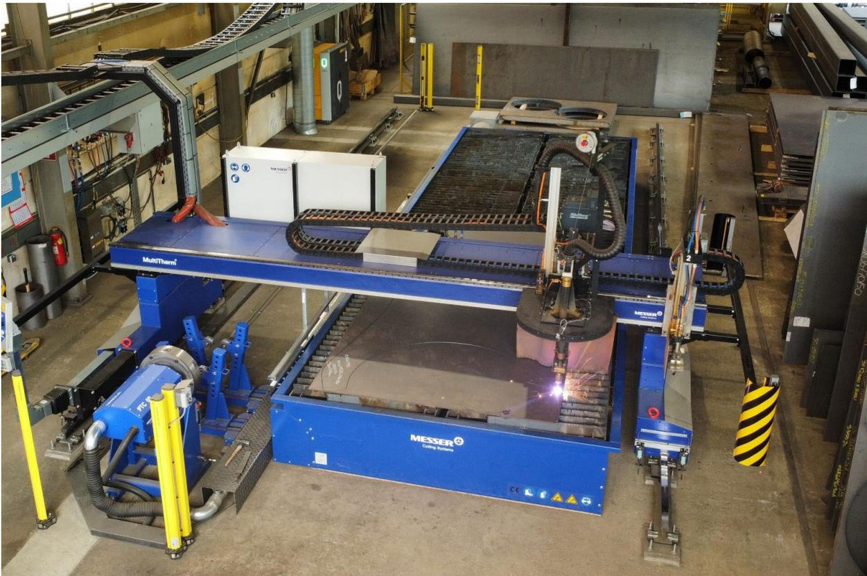
**Caption 2:** The new MultiTherm cutting machine from Messer Cutting Systems with plasma bevel unit, ALFA oxyfuel torch and pipe cutting system. © Thöni Industriebetriebe GmbH
